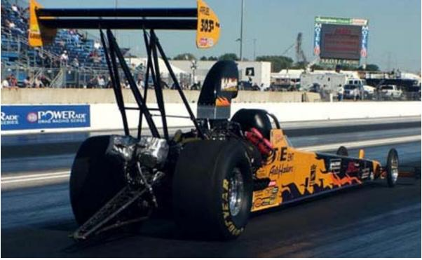
2001 MCKINNEY 298" CHASSIS – LAST RAN FALL OF 2008 BAE ENGINE BLOCK – 4.375 BORE –  $\frac{1}{2}$ " DECKED – RAISED CAM – 433 C.I. MOROSO OIL PAN BRYANT 3600 CRANK BME RODS
